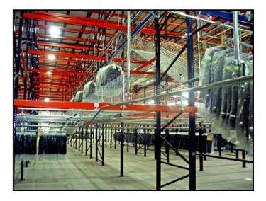
This means that the trolleys can be stopped, switched or diverted to other paths (powered or non-powered). The system design can enable trolleys to accumulate with one another anywhere within the system. This provides positive control of the trolleys at all times and allows for a wide variety of functions/process to be performed.
